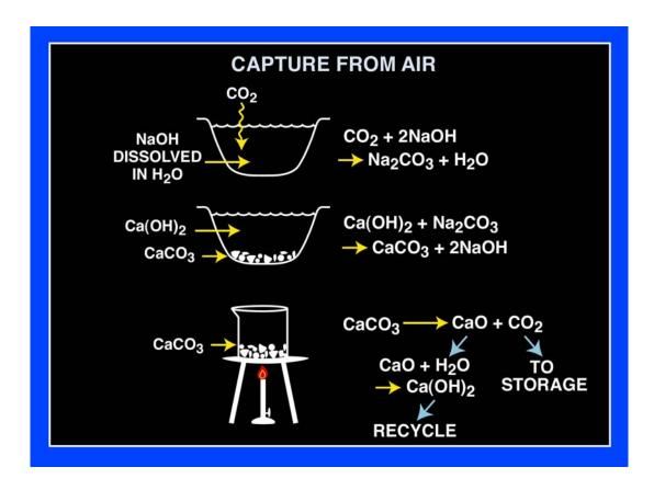
**Figure 57.** CO<sub>2</sub> is readily absorbed in basic solutions such as sodium hydroxide. It can then be recovered by adding calcium oxide or calcium hydroxide to the sodium hydroxide and thereby precipitating calcium carbonate. The calcium carbonate is then separated from the sodium hydroxide and heated in a kiln. At 900°C, the CaCO<sub>3</sub> dissociates into calcium oxide and CO<sub>2</sub>. The calcium oxide is recycled. The CO<sub>2</sub> is liquefied and piped to the storage site.
